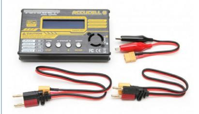
The Accucel 6 Balance Charger utilizes quality FETs and resistors to accurately balance and charge LiPoly, LiFe, LiHV, NiMH, NiCd, and Pb batteries. If you are looking for a charger for your Bolt or any other LiHV batteries this unit is perfect as a low-cost solution. The Accucel-6 will handle LiHV/LiPoly/LiFe up to 6S and NiMH/NiCd up to 15S and shows individual cell voltage throughout the charge cycle.
